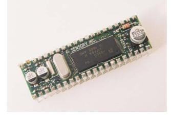
Using the VR Stamp<sup>™</sup> Toolkit, application programs can be downloaded into the VR Stamp. The VR Stamp can then be removed from the Module Programmer Board and plugged directly into the final product. In-circuit reprogramming is also supported.
